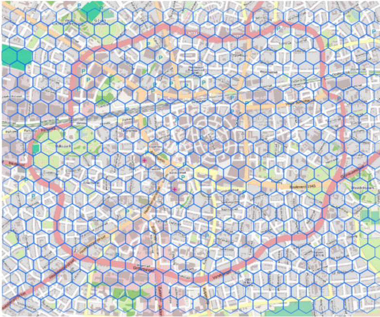
Figure 6.7: OpenStreetMap of Enschede centre overlaid with a hexagonal tessellation of cell size around 70 meters
